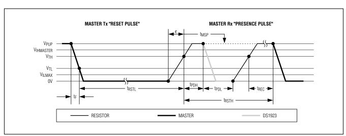
Figure 12. Initialization Procedure: Reset and Presence Pulse
