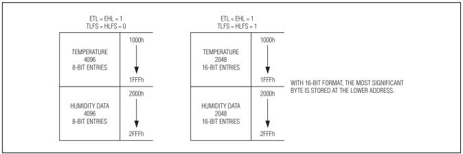
Figure 7b. 2-Channel Logging, Equal Resolution
