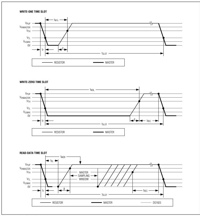
Figure 13. Read/Write Timing Diagrams
