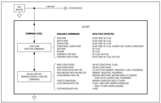
Figure 2. Hierarchical Structure for 1-Wire Protocol
