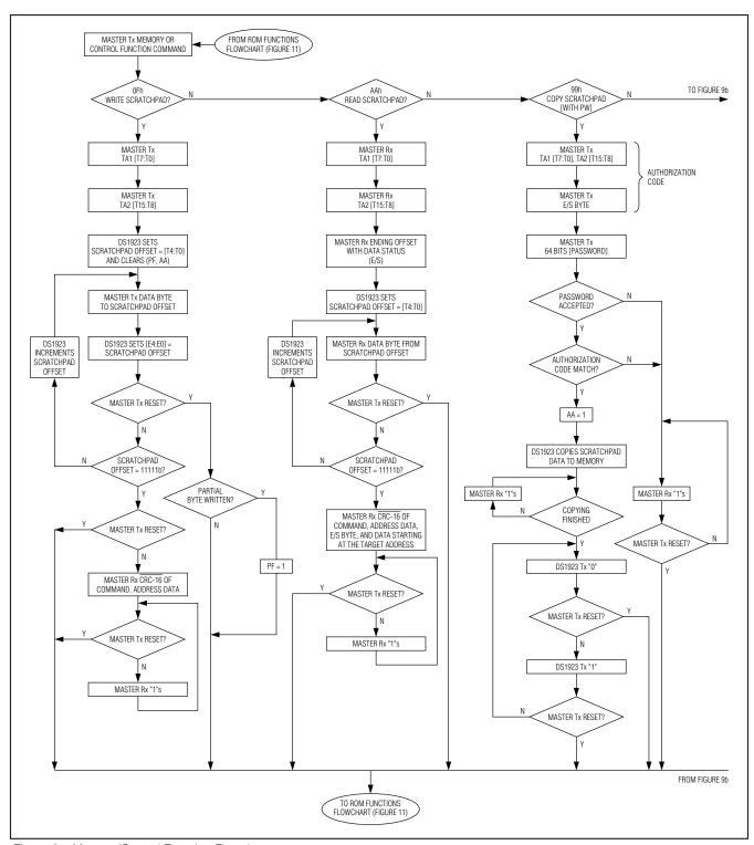
Figure 9a. Memory/Control Function Flowchart
