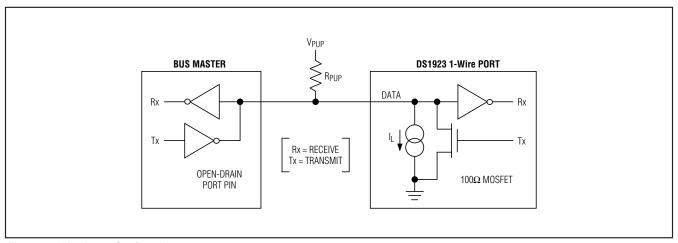
Figure 10. Hardware Configuration
