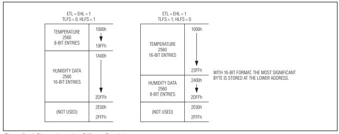
Figure 7c. 2-Channel Logging, Different Resolution
